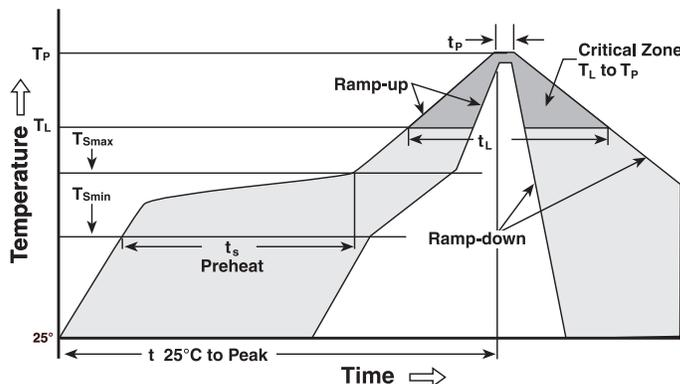
Figure 5. Typical reflow profile
