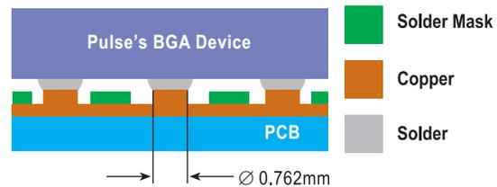
**Figure 3.** Recommend Land Pad for BGA device
