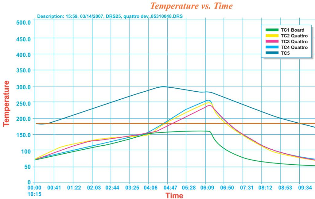
Figure 7. Quattro/Dos Lead-free, Thermal Plot (lead-free devices)
