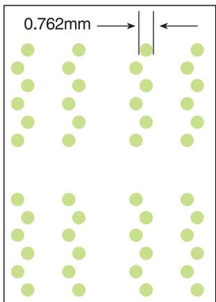
Figure 4. BGA device stencil example
