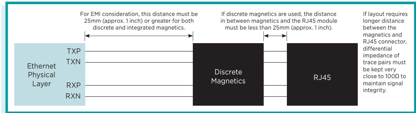
**Figure 1. Pulse Ethernet Magnetic and RJ45 Placement**
