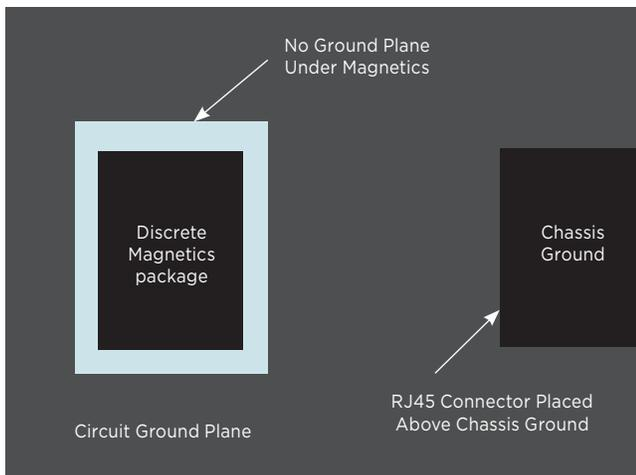
**Figure 6. No Ground Planes Beneath Discrete Magnetics**
